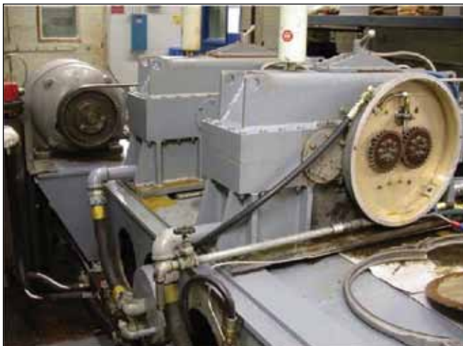
Figure 13—Scuffing test rig with cover removed and test specimen gears installed.
