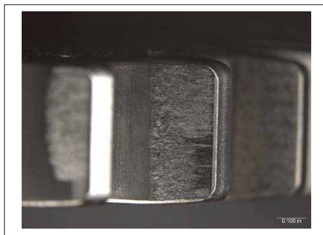
Figure 18—Close-up view of a representative scuffed tooth.
