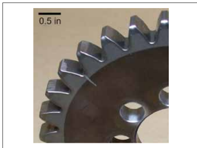
Figure 17—Scuffing failure of baseline test gear.
